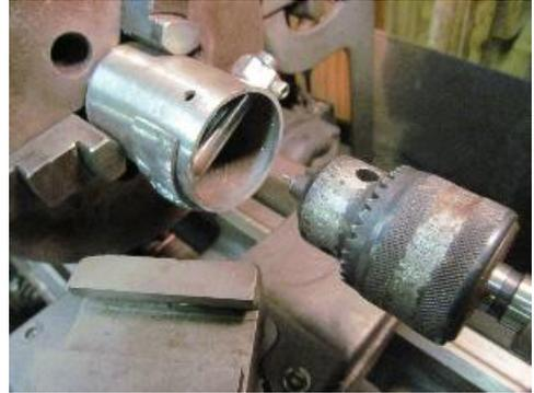
The switch to the #60 bit and micro-precision drill chuck and make the hole (very gently!).
