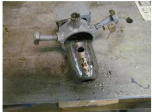
To insure that the holes are aligned, the bell is inserted and rotated past the bottom hole. When a 1/4" pipe section can be inserted through the hole and into the bell, the bell can be locked in position and the second hole generated as described above.
