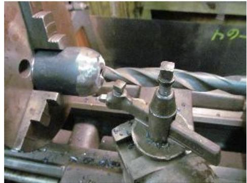
The last operation is to face the bottom to create a flat area surrounding the opening. This will be the seat on which the 3/4" down pipe will be welded.
