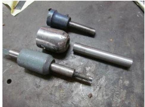
Just slide the components together, tack weld one position, rotate 180 degrees and start running a complete bead around the junction of the bell and the down pipe.
