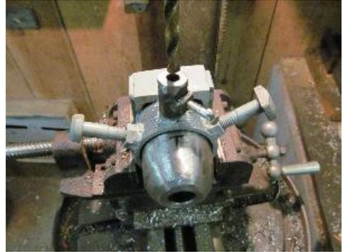
The small drill adapter is removed and the bit replaced with a 3/8" bit. It is then run through the wall of the bell. Cooling fluid does help if available.
