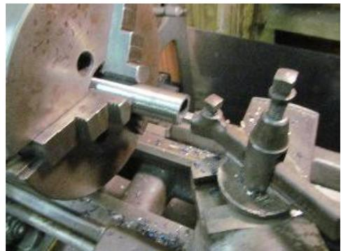
If the down pipe is to eventually slip into a section of 1" pipe, you can either reduce the exterior diameter of the down pipe (by  $\sim 0.020''$ ) or bore out the diameter of the 1" pipe. The first is actually easier and this step can be done after the bell is welded to the down pipe. Note the use of a bull nose live center.
