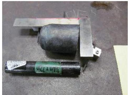
But first the bottom was ground a bit on the 2x72 knife grinder to remove any major wrinkles and to create a quasi-flat on the bottom (as shown). The next task is to face the opening.
