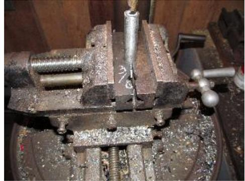
Take a piece of 3/8" round scrap, grind a bevel on one end and then saw off that end to generate a plug ~ 1/2" long. Tap it into the non threaded end of the nipple and position the strap as shown. All that is needed is to weld the plug over the entire 360 degrees and weld the strap to the pipe.
