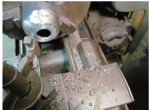
Face the down pipe on both ends.
