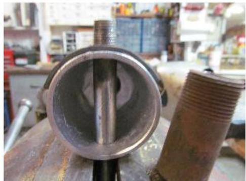
Since the gas pipe is one of the more expensive items in this build, you can just buy a 4" nipple or an 8" nipple and saw it in half. Either way, you want a length that spans the bell plus ~0.5" (not including the threaded section). Run a 3/8" bit into the pipe for maybe 1/2".
