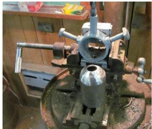
The process starts with slipping a small drill (letter size "T") adapter over the top pipe and running the 'T' bit through the side of the bell clamped in the jig.
