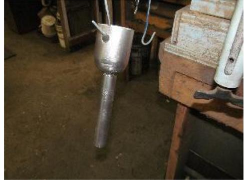
What is left is the fabrication of the gas pipe and that includes precisely drilling an orifice in the dead center of the bell. This starts with the creation of a strap that wraps part of the exterior of the bell and that starts with a pilot hole – here an 1/4" hole centered in the 1" x 1/8" x 3" flat stock.
