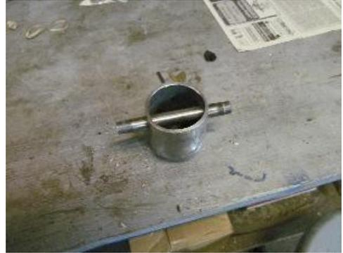
The down pipe needs to be welded to the bell so that it is dead straight and aligned with the hole in the bell. This is most easily done with another jig. It can consist of the drill adapter slug and a piece of round stock that will fit the ID of the down pipe. I happened to have the lock mechanism from a weight lifting bar in the scrap bin, so a few seconds on the lathe made essentially the same thing.
