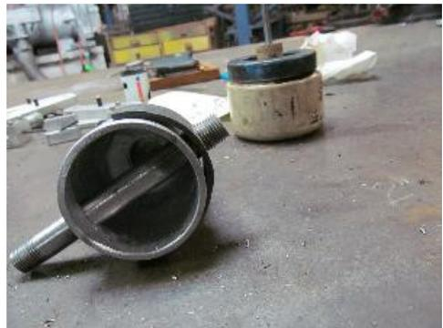
So clamp the assembly in a machinist vise and use a trashed pipe section inserted over the tube and a hammer blow or two to correct any discrepancy in the fit.
