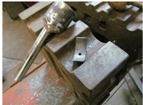
Use a 13/64 bit and drill the strap so as to accommodate the gas pipe.
