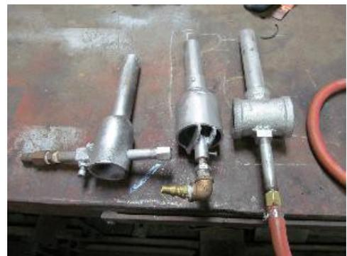
The bell burner version can easily be turbo-charged by adding axillary air pressure provided by a small blower. Shown here is a manifold that locks onto two bell burners and is powered by a small squirrel cage. At 10 psi, this forge easily exceeds 3000 F which is why there is a slide gate on the air line to prevent melting the refractory. This particular forge was designed for welding pattern-welded steel and has been in service for better than 10 years without touching the burners.
