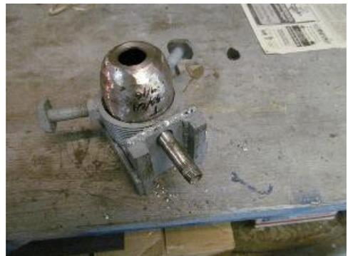
If all goes well, a gas pipe now runs through the center. Any drill flash should be removed with the air die grinder.
