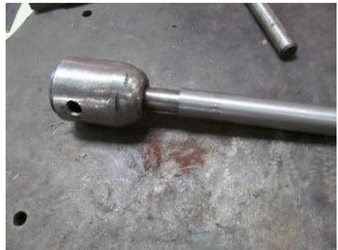
After the weld, clean up on the knife grinder and...
