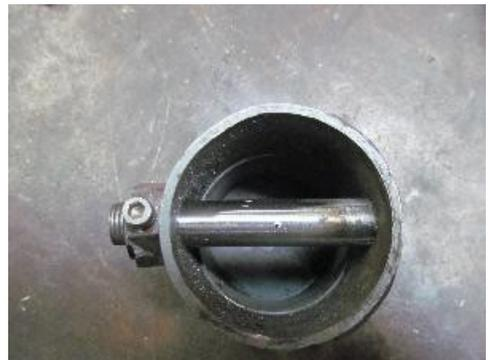
So invert the gas pipe (orifice has to pointed down the down pipe and not in your face), clamp it in place and tack weld the ends of the strap.
