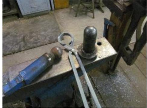
The bell is run up to forging temperature, dropped on the mandrel and then hammered to force the bell to approximate the mandrel's 2" hemispherical shape. The neck formed by sawing the sections apart is driven down as shown. What is critical is the interior of the unit, so some wrinkles on the outside can be tolerated.
