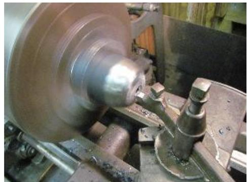
The idea is to enlarge any opening sufficiently to allow the drill bit not to wander.
