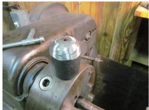
The goal is to position the bell in the three-jaw chuck as close to square as possible. I found that using a 13/16 drill bit and an alignment slug (more on this later) inserted into the bell acts as a rough bull-nose live center to align the unit. Once the chuck is closed, the tail stock is slide out of the way and the bell edges are faced.
