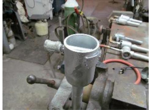
If needed for hitting welding temperatures, add a small blower (15 cfm seems sufficient in my forge).
