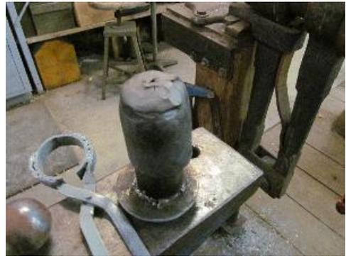
One possible problem with the saw cut is shown here – the opening of the bell is not perpendicular to the sides. That has to be fixed, so it is time to visit the machine room.
