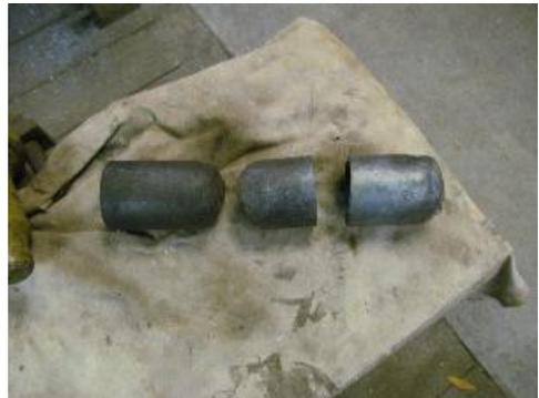
The next step is to forge the bells as smooth and radially symmetrical as possible. The tools consist of a set of tongs that can easily grip the 2" pipe sections and a mandrel. The first one I built used a 2" trailer ball welded to some round stock. The current one uses a 2" ball bearing welded to a 1.5" pipe section. Both were equipped with a hardy stub for my anvil.
