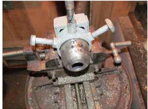
Hole Number one is done. The bell needs to be rotated 180 degrees and the drilling procedure repeated.
