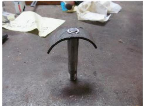
After a good deal of experimentation with MIG tips and 1/4" pipes, I have decided that drilling a hole is far superior. You need a #60 (0.040") or #65 (0.035") wire drill (about \$0.85 from Enco – you will have to buy a dozen which -of course- insured that you will never break a bit). Add a precision drill chuck (Enco stock # 891-5837 < \$10) and you are ready to make a hole.
